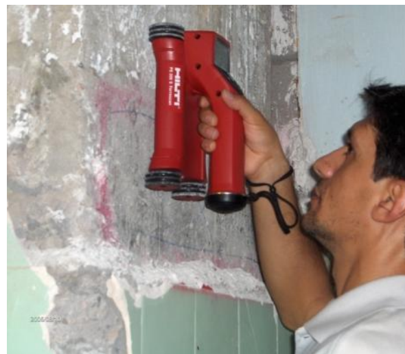
Non Destructive Tests to evaluate the existing structure. Staffs locating the rebars in the structural elements. Bandar Abbas, Iran 10/08/2005
