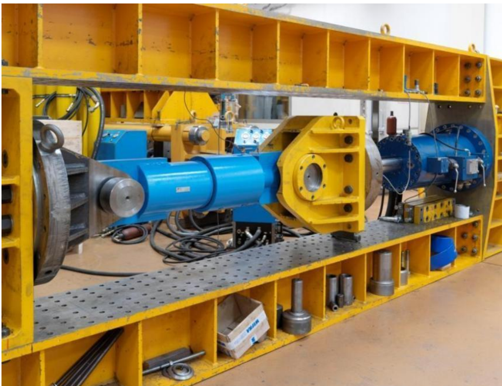
One of the hydraulic Dampers installed in the test setup to measure the technical characteristics under supervision of Swiss Federal Institute EMPA expert Dr. Felix Weber. FIP Industriale, Padova, Italy 07/03/2008
