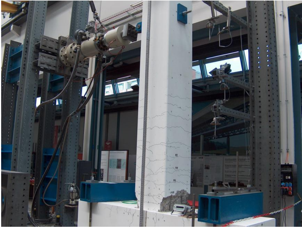
Prototype RC column to simulate Azadi Grand Hotel rectangular RC columns under cyclic earthquake load prior to design phase. Empa structural labs, Zurich, Switzerland 02/22/2005
