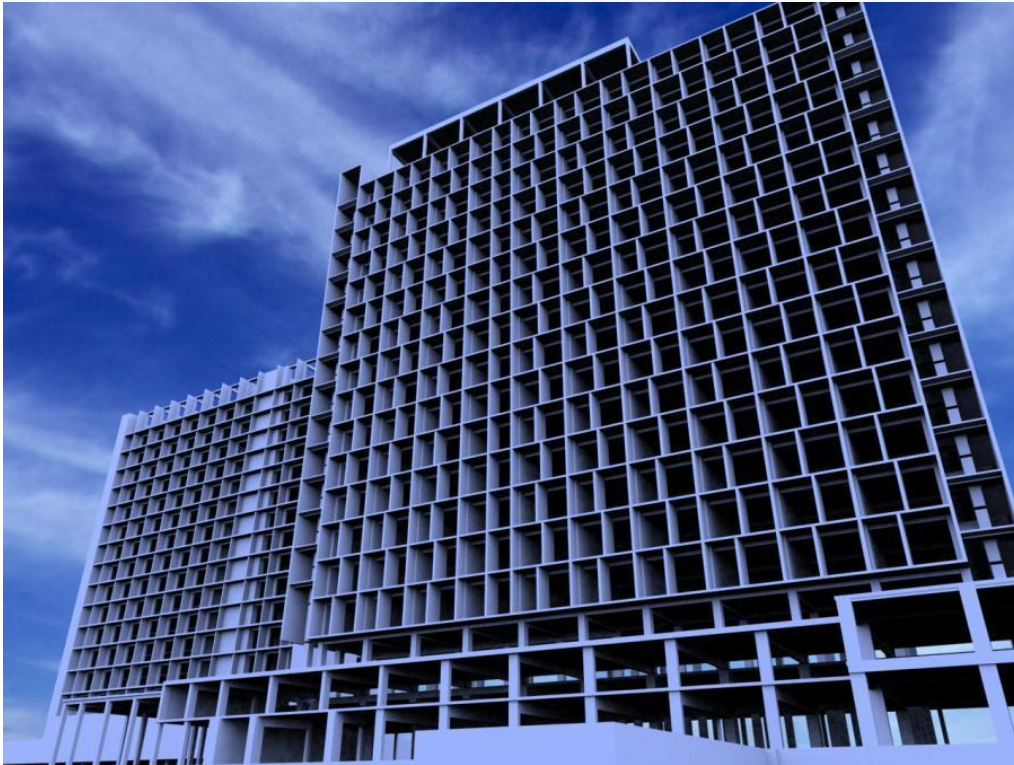
As Built 3D Structural Model of the building based on the detailed study is provided for Dynamic Analysis of the building in ADINA program. Radyab Co. Tehran, 2005
