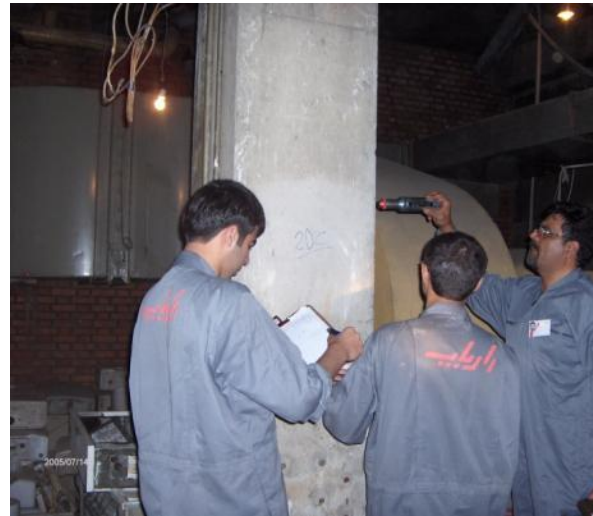
Non Destructive Tests to evaluate the existing structure. Left picture: Locating the rebars in the building foundation. Right picture: Determining concrete compressive strength by means of Schmidt Hammer. Esteghlal Hotel, Tehran, Iran 07/14/2005
