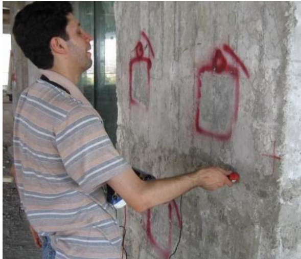
Non Destructive Tests to evaluate the existing structure. Ultrasound Wave Transducer to determine concrete consistency (left). Locating the rebars in the building structural elements by Rebar Locator (right). Bandar Abbas, Iran 06/28/05
