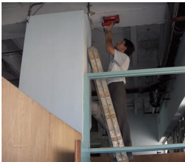
Non Destructive Tests to evaluate the existing structure. Staffs locating the rebars in the structural elements. Bandar Abbas, Iran 10/08/2005
