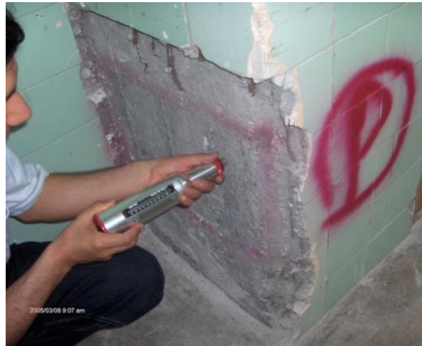
Non Destructive Tests to evaluate the existing structure. Determining concrete compressive strength by means of SCHMIDT Hammer. Bandar Abbas, Iran.08/03/2005
