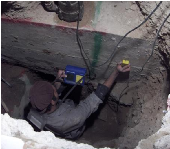
Non Destructive Tests to evaluate the existing structure. Left picture: Locating the rebars in the building foundation. Right picture: Determining concrete compressive strength by means of Schmidt Hammer. Esteghlal Hotel, Tehran, Iran 07/14/2005
