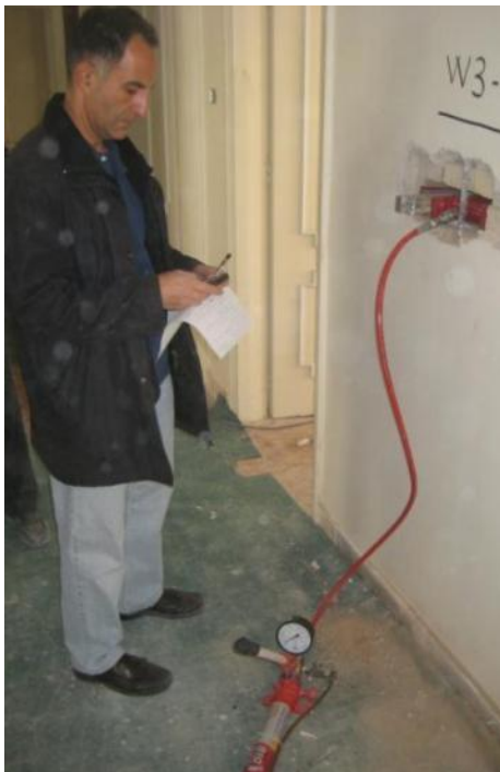
Professor Motavalli (Empa) checking the Masonry Shear Test setup (left) and discussing the structural details with Radyab Co. staff (right). Tehran, Iran 05/12/08
