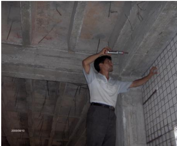
Non Destructive Tests to evaluate the existing structure. Determining concrete compressive strength by means of SCHMIDT Hammer. Bandar Abbas, Iran.08/03/2005
