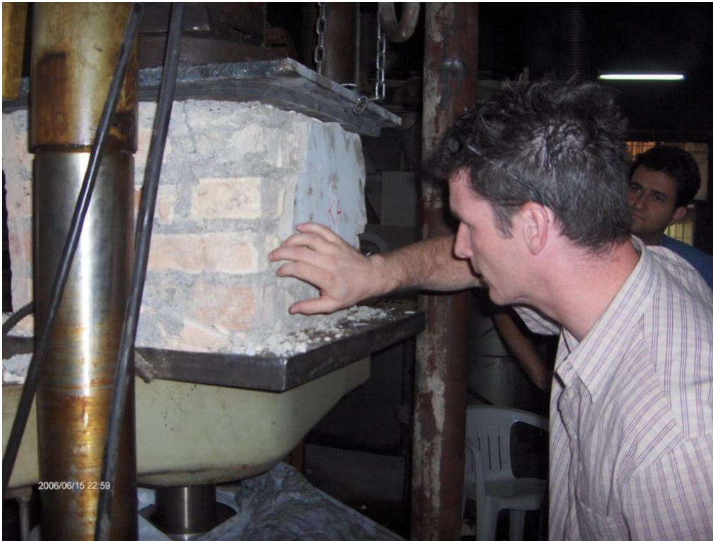
Compression test to be carried out on a masonry wall specimen taken out of load bearing walls in Swiss Embassy Building. Supervisor: Mr. Sven Heunert. Amirkabir University, Tehran 06/16/2006
