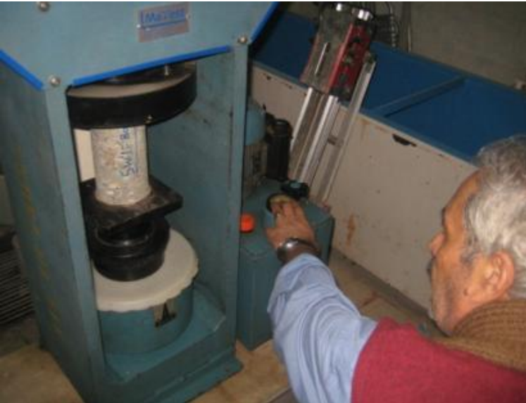
Compressive tests to check the shear walls concrete quality. Tehran, 12/24/2008
