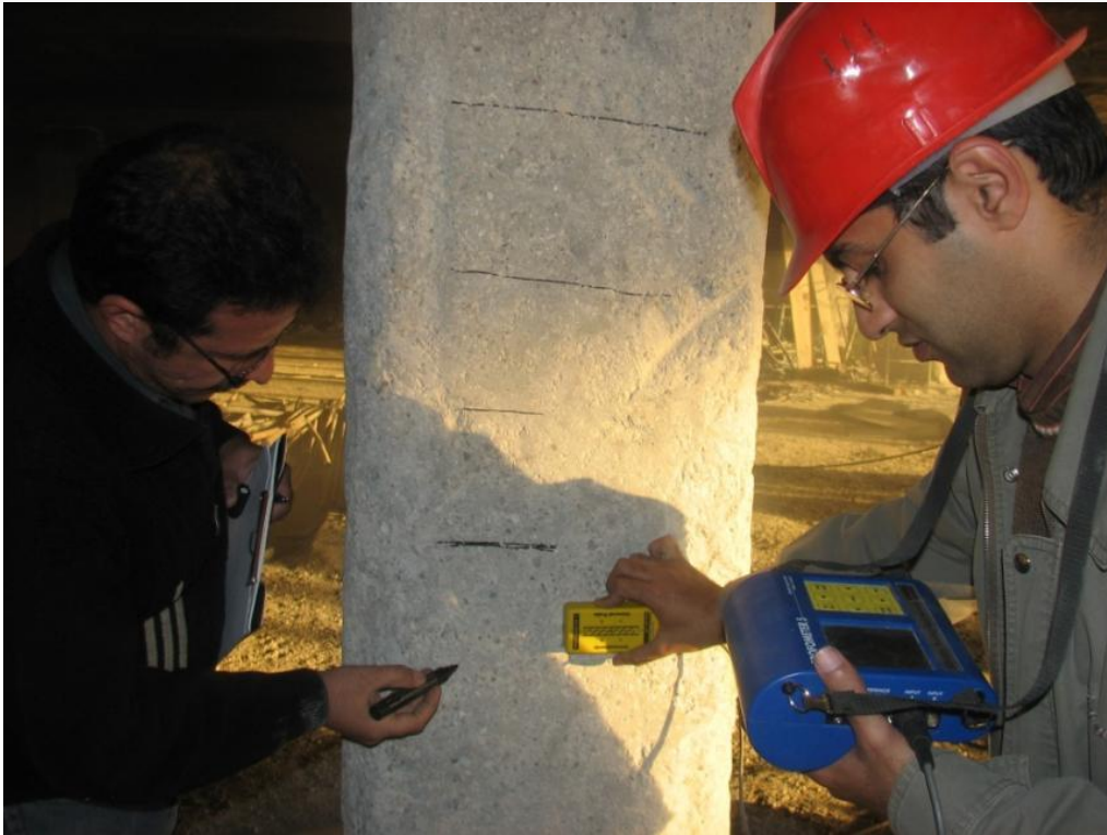
Radyab staff determining the rebars inside the RC columns by means of Rebar Locator Scanners in Structural Evaluation phase. Tehran, Iran 11/16/2007
