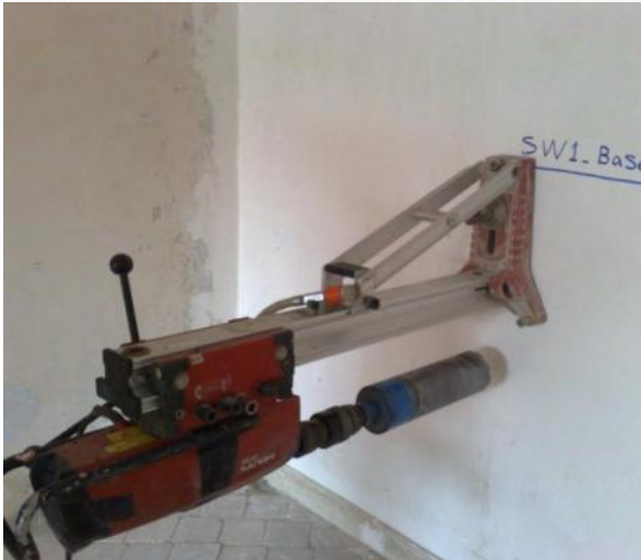
DT Tests (Concrete Core) to check the shear walls concrete quality. Tehran, 12/03/2008
