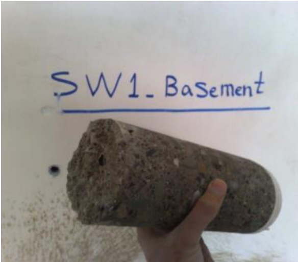
DT Tests (Concrete Core) to check the shear walls concrete quality. Tehran, 12/03/2008
