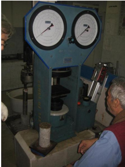
Compressive tests to check the shear walls concrete quality. Tehran, 12/24/2008
