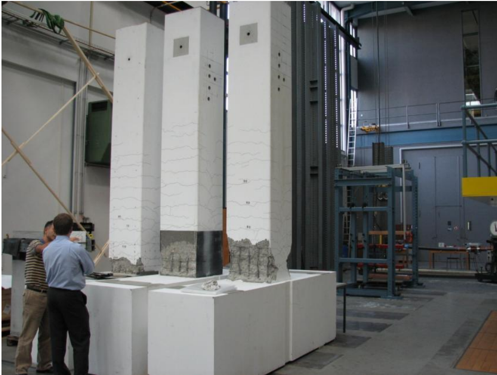
Three different prototype RC columns under cyclic earthquake load prior to design phase. Empa structural labs, Zurich, Switzerland 09/20/2006
