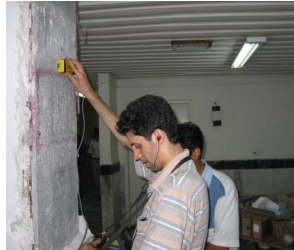
Non Destructive Tests to evaluate the existing structure. Ultrasound Wave Transducer to determine concrete consistency (left). Locating the rebars in the building structural elements by Rebar Locator (right). Bandar Abbas, Iran 06/28/05
